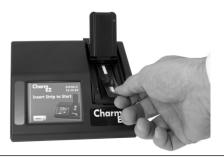
Within 3 minutes of completing incubation, insert clean and visually valid test strip into Charm EZ system as shown. Slide test strip completely into slot until it stops.
